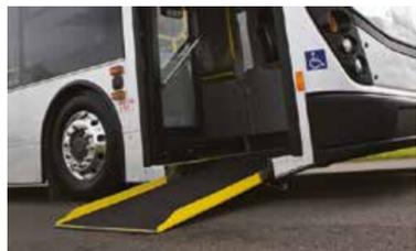
Low step and flat floor allows full access for wheelchairs.
